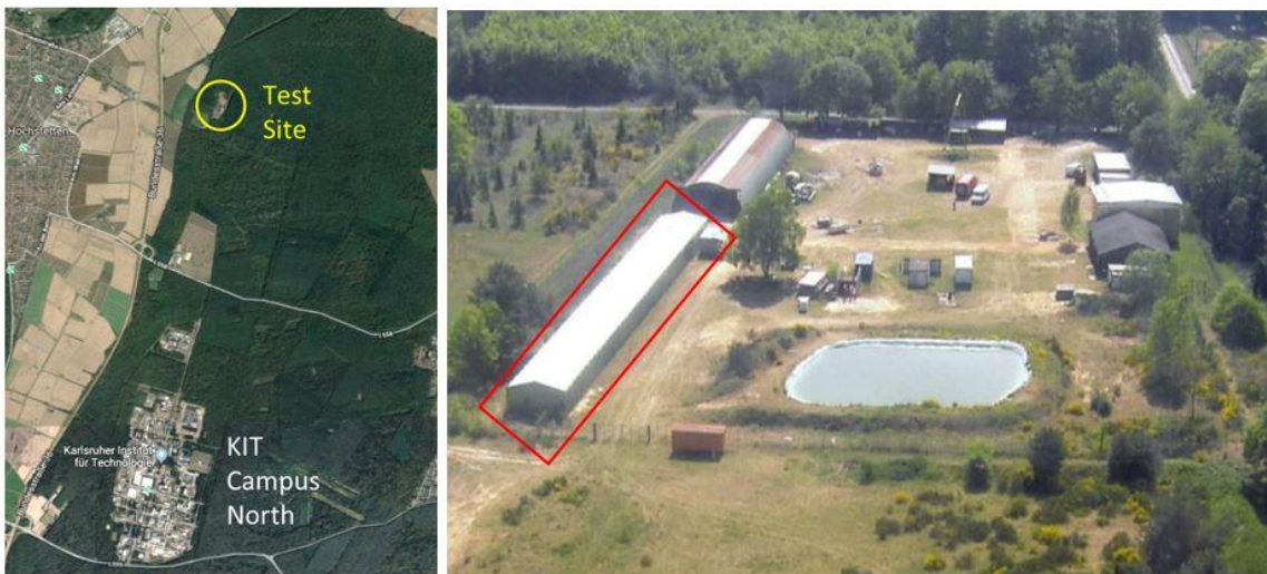
Figure 15: Location (left) and aerial view from the north (right) of the free-field test site north of KIT Campus North with position of the concrete pit (red rectangle).
