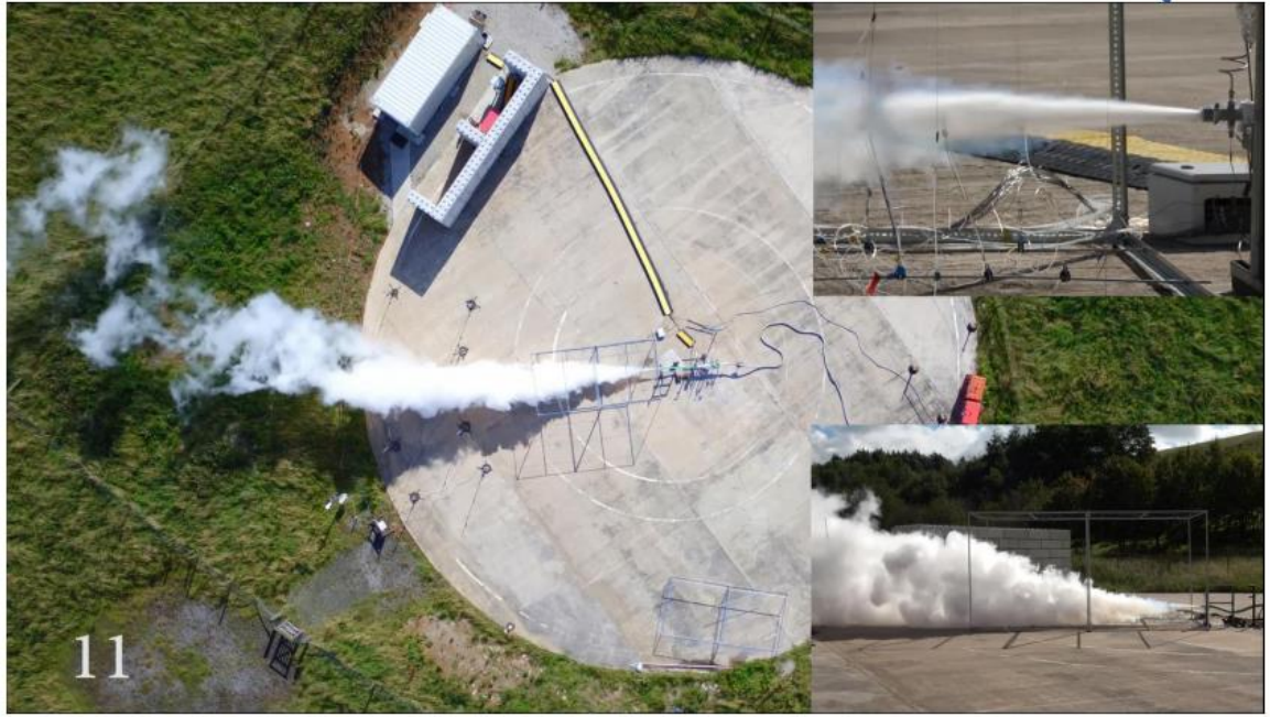
Figure 9: LH 2 large-scale release (HSE, test realized within PRESLHY).
